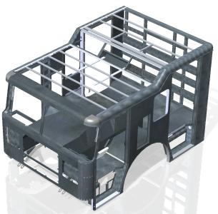
**Cab Safety Cage Specifications:** Roof Assembly: 1.25" Stainless Steel Tubing Front A Pillar: 2"x3" Stainless Steel Tubing Back Wall: 1.25" Stainless Steel Tubing Sides: 1.25" Stainless Steel Tubing 142" Attacker ® / Split Cab
